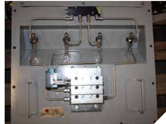
Metered lubrication is precisely applied to the teeth
