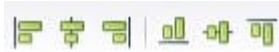
Fig. 50. Align. With this toolbar the user can align selected units in many ways, thus making it easier to draw professional-looking flowsheets.
