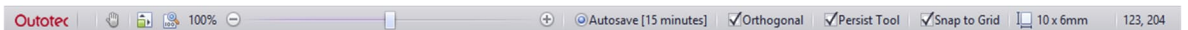
Fig. 55. With the status bar the user can fit and zoom the flowsheet and check and uncheck the Orthogonal, Persist Tool, Autosave, and Snap to Grid options. If the user wants to draw Orthogonal streams or lines (see Fig. 45 and Fig. 47 ), check this option. The Persist Tool remembers the last used drawing tool so that the user does not have to select the same tool again separately. The Snap to Grid option aligns the streams and units according to the grid on the flowsheet, thus making it easier to draw professional-looking flowsheets. The user also sees the size of the chosen object and position of the mouse cursor.
