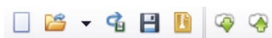
Fig. 56. With this section of the top toolbar, user can start a new or open an old process. It is also possible to save the process, save a backup, a zip file (archive) of the process or use the Model Base to download or upload models.
