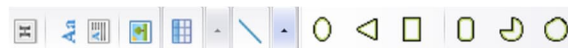
Fig. 47. Drawing tool. With this toolbar the user can draw a line, add shapes like an ellipse, a rectangle, a rounded rectangle and so on. It is also possible to add a header, text label, a text box, a picture and a table.
