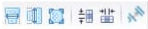
Fig. 49. Height and Width. With this toolbar the user can make the size or spacing of the selected units or streams equal. At least 3 units are needed for equal spacing of the units.
