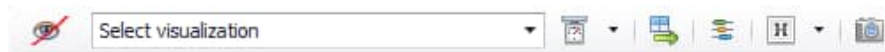
Fig. 46. Visualization. Select or deselect the visualization mode and select the stream property that is visualized. The user can also change measurement units, open the Stream Table Editor, visualize stream connections, add a header, and copy the flowsheet image to the clipboard using this toolbar.
