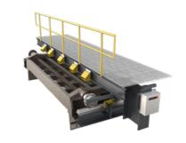
To provide accurate, real-time information about the pallet condition during operation and thus clear criteria for service intervals, Metso Outotec has developed its condition monitoring system. The system consists of a Pallet Car Identification System via optical cameras or RFID, a Sag Monitoring for the pallet bodies with contactless sensors and further sensors to detect missing grate bars or wheels.
