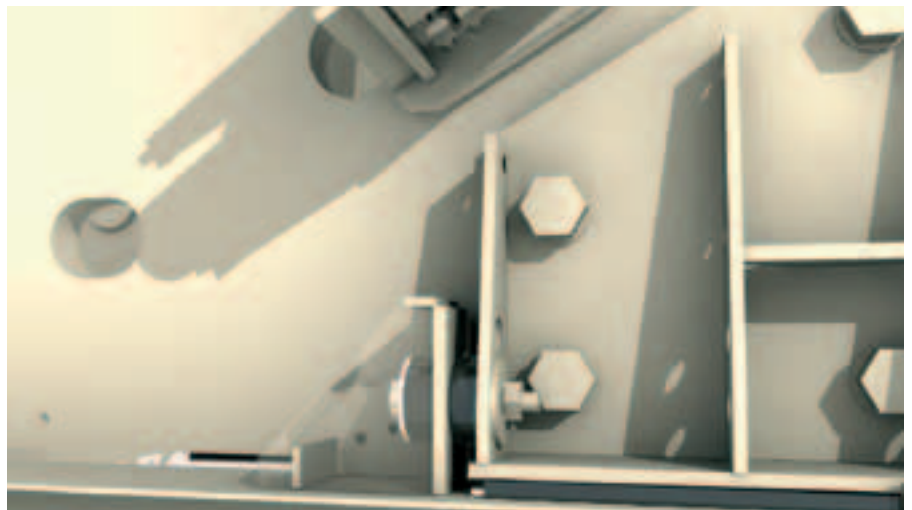
Special rubber dampers and stoppers allow the crusher to move vertically and longitudinally while preventing wear and subsequent damage to the crusher's foundation.
