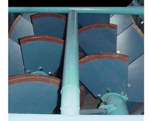
Mixer conditioners are designed for ash handling applications. Mixer conditioners will help simplify the final transfer of material to the storage facility or location by wetting the ash.
