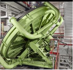
The green pellet size measurement system VisioPellet™ is a continuous real-time expert level process assessment that optimizes pellet size distribution and feed rate. This is the basis for a real pellet size control loop, optimizing disc speed and inclination, water addition and feed rate.
