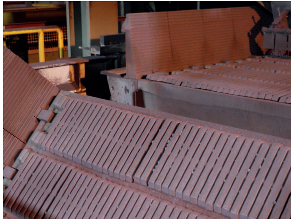
Metso pallet cars are used in pelletizing furnaces with reaction areas from 180 to 816 m 2 and with a grate factor of up to 28 tons of pellets per day and m 2 for hematite and 40 tons per day and m 2 for magnetite ores.
