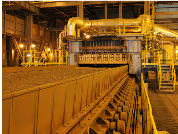
The easy to maintain sidewalls ensure that the feedstock remains on the pallet car. Our pallet cars are used in sintering machines with reaction areas up to 600 m 2 , with a grate factor of up to 45 tons of sinter per day and m 2 . Sinter bed heights up to 730 mm can be achieved.
