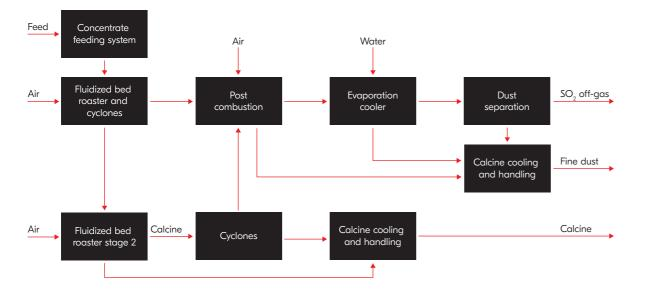
Our two-stage roasting plants are mainly used for treating double-refractory gold concentrates. A two-stage roasting process combines partial roasting in the first stage with dead roasting in the second stage. The first stage is used as a de-arsenifying process step in an oxygen-deficient roasting atmosphere, while the second stage operates in an oxidizing atmosphere to fully transform the metals into their oxide form.
