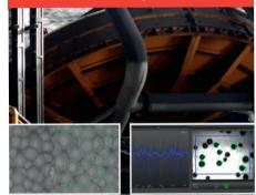
VisioPellet™ is a real-time expert level process assistant that optimizes green pellet size distribution and feed rate.
