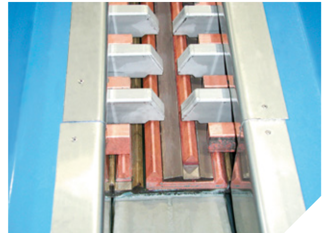
Patented DoubleContact™ busbar system ensures more even cathode weight distribution.
