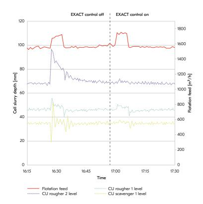
ExactLevel is also a built-in functionality in Metso CellStation flotation cell controller
