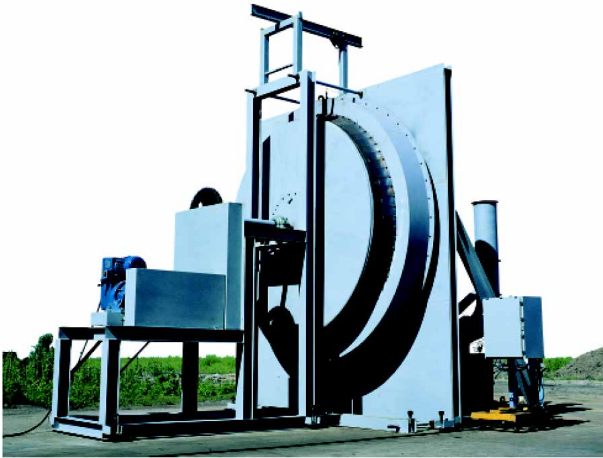
Metso Outotec 10' test unit used for the development and continued improvement in air seal design
