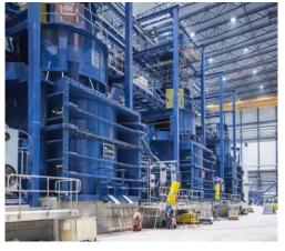
Several energy-efficient stirred mills to a greenfield iron ore processing plant
