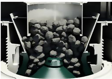
Good feed material level
