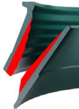
Example of normal wear. Obtained with correct feed arrangements, feed gradation and parameters for the cavity.
