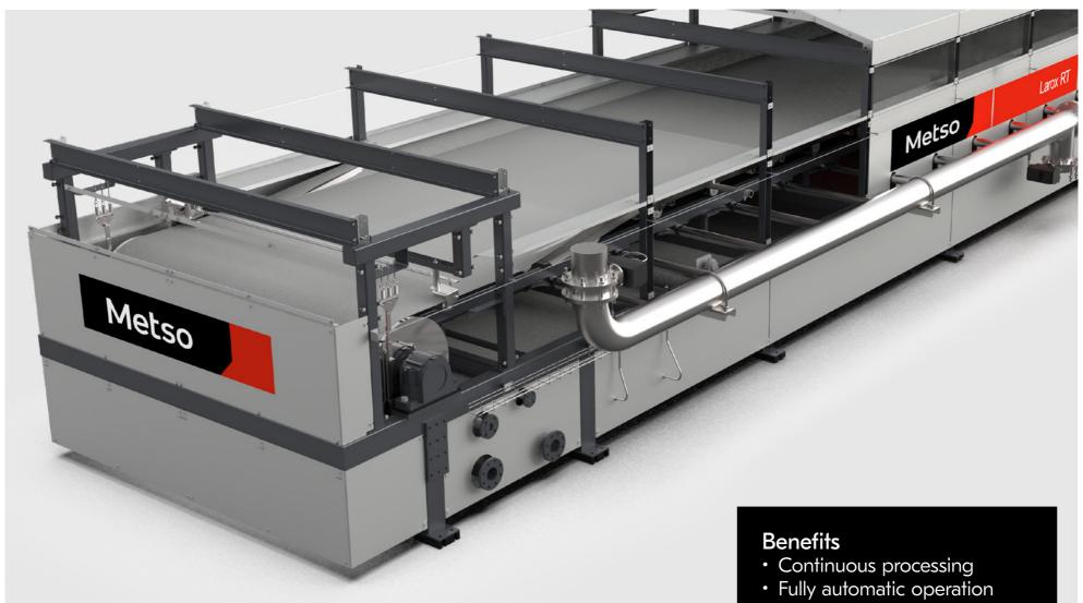
Metso Larox® RT (Reciprocating Tray) belt filters utilize a totally unique design proven over 50 years, the filter offers true multi-step processing in a single unit. The processing capabilities include superior cake washing in either co-current or counter-current modes and enhanced dewatering through cake vibration, mechanical compression or thermal drying.
