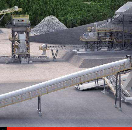
Using the latest technologies, the RockSense™ portfolio products enable continuous and accurate online information regarding the on belt coarse particle size distribution.
