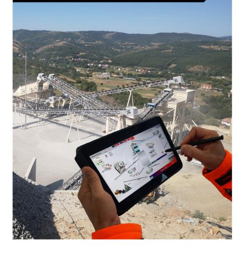
Metso introduces newly branded Controlled Aggregates & Mining Efficient Operation System (CAMEOS), which combines simplicity, availability, optimized regulations and comprehensive message history to help maintain crushing and screening plants.
