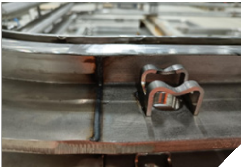
Laser welded seam
