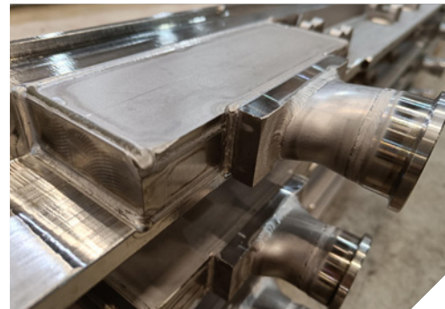
Laser welded seam
