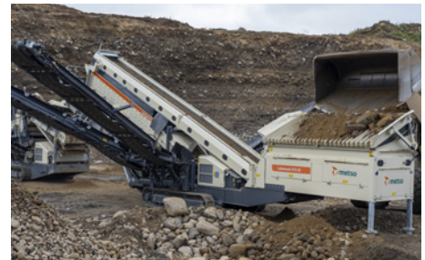
Large feed box allows closed circuit process.
