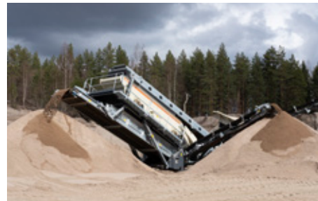
Adjustable conveyors for high stockpiles.
