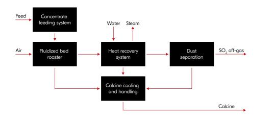
Dead roasting is the most commonly used roasting process and is mainly applied in our zinc and pyrite roasters. When using a dead-roasting process for concentrates, the sulfides are completely transformed into oxides. The gas temperature in this type of plant is typically between 800 and 950°C. The hot gas generated in the process is used for heat recovery and is suitable for high-pressure steam production in a waste-heat boiler.
