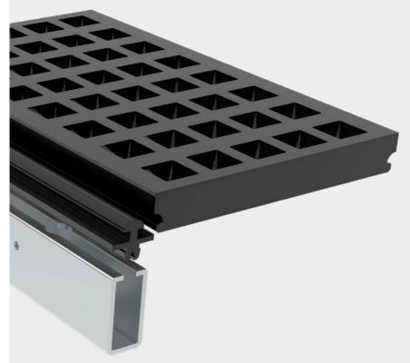
Designed for the aggregate business with focus on stationary plants. Compatible with well-known and proven aggregate industry standard fixing systems. Configurable to support all applications. Trellex® GS is designed to increase uptime and safety. The modular screening media with knock-in system is available in both rubber and polyurethane to offer long wear life and flexibility.
