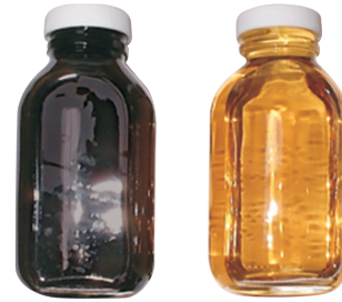
Dirty and clean oil samples, before and after oil filtration. The filter inserts have absorbed the contamination from the crusher oil, and an oil change has now been avoided.
