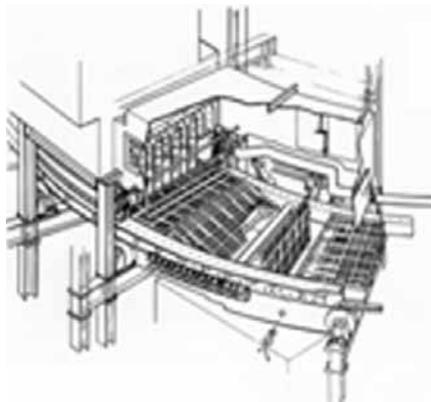
Shows the pallets tipping to discharge the pellets.
