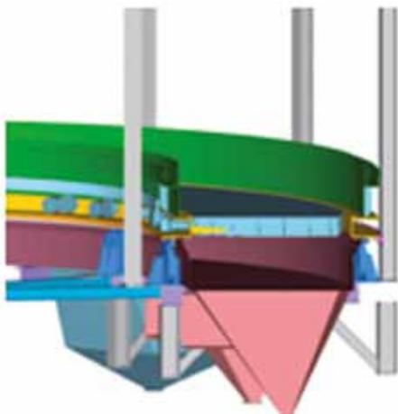
Side view of the pallets that carry the indurated pellets
