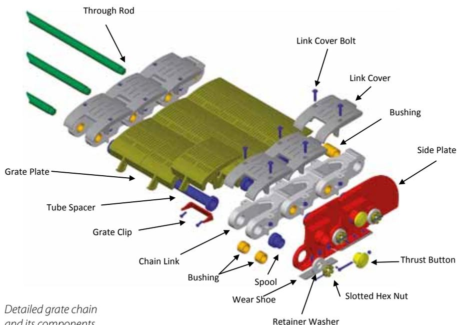
Detailed grate chain and its components
