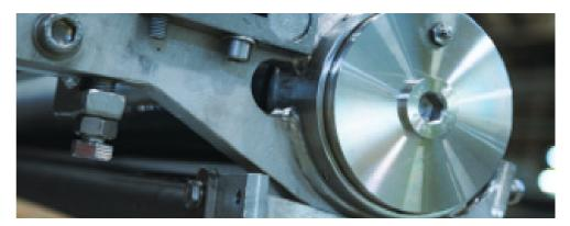
Filter rollers are responsible for driving, steering, tracking and tensioning the cloth.
