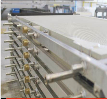
Plastic PF filter plates are the best solution for extremely corrosive applications in industrial filtration.
