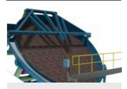
The green pellet size measure-ment system VisioPellet™ is a continuous realtime expert level process assessment that optimizes pellet size distribution and feed rate. This is the basis for a real pellet size control loop, optimizing disc speed and inclination, water addition and feed rate.
